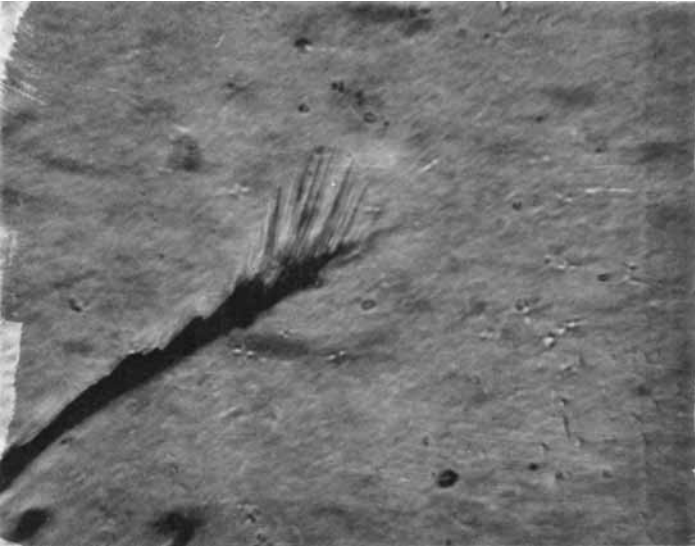
Fig. 6. Termination of crack in blend 85/15-4 (620 \times ).
